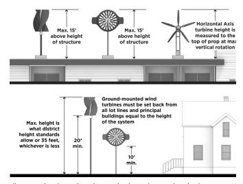
Illustration of regulations for roof-mounted and ground-mounted wind turbines
